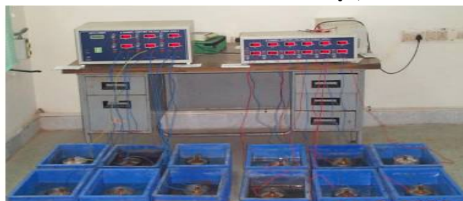
Figure 2: Concrete Elements Set for Polarization Study (Accelerated Corrosion Test)
