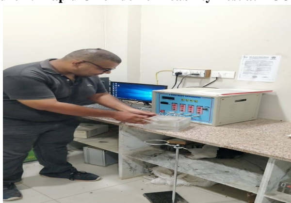
Figure 1: Rapid Chloride Permeability Test at RCC Lab
